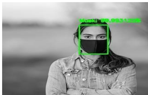
Figure 5.1: When The Person Not Wearing the Mask . A bounding box drawn over the face of the person describes weather the person is wearing a mask or not. If a person’s face is stored in the database, it detects the name of the person who is not wearing face mask.
