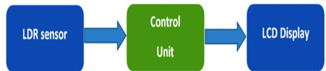
In the receiver section, the LDR sensor receives the visible light pulses from the transmitter side and converts it into interpretable electrical pulses, which is fed to the Arduino (Control unit). Arduino receives this pulse and converts it into actual data and displays it on a 16x2 LCD display.
